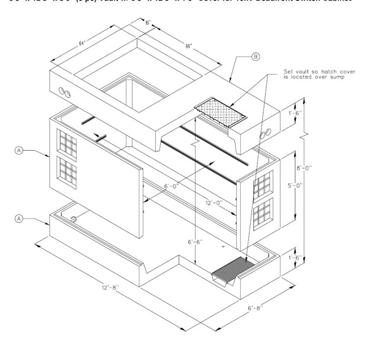
782202.1 6'8 x 12'8 Precast Concrete Vaults and Associated Pads and Covers
